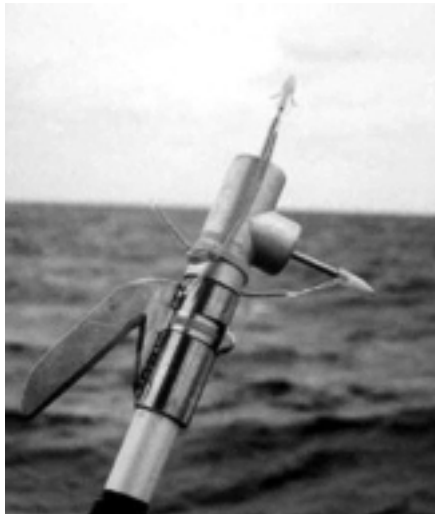
Figure 9. Dual applicator tagging pole, with a perpendicular as well as parallel applicator, used to improve the accuracy of tag placement into giant bluefin tuna caught off Hatteras, North Carolina (see text).
