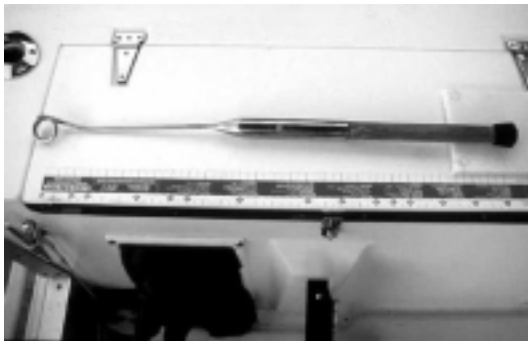
Figure 20. Commercially available de-hookers are very effective in removing "J" hooks from large highly migratory species.
