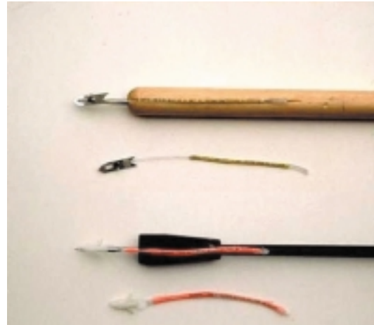
Figure 2. Stainless steel dart tag, Tag A (top) and hydroscopic nylon double-barb dart tag, Tag B (bottom) used in the double-tagging study to evaluate retention of the two tag types on billfishes (1990–1999).
